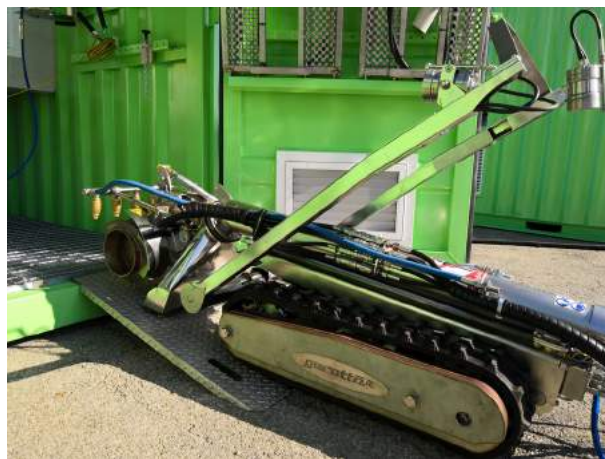
Figure 2. Example of a tracked mini crawler to be attached to a suction machine.
